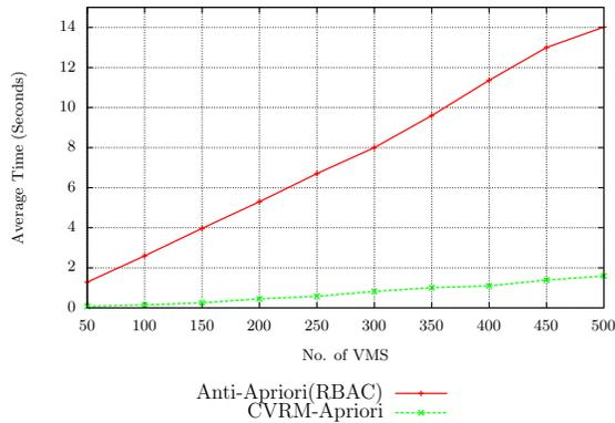
Figure 8: Mining Time with Increasing No. of VMs
