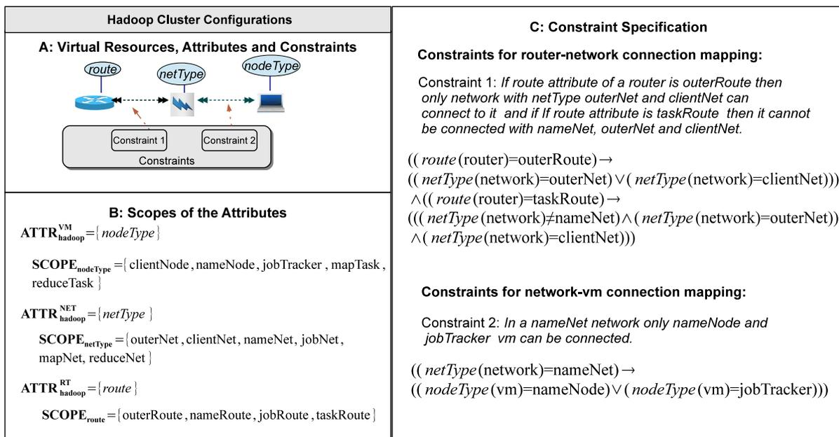
Figure 10: Constraints Specification for Hadoop Cluster
