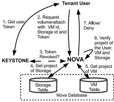
Figure 5: Operation *volume-attach* in Nova
