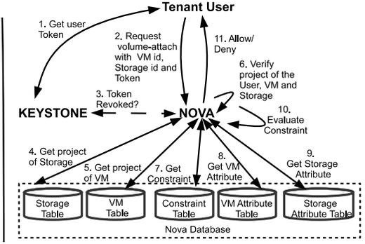
Figure 7: Constraint Enforcement for *volume-attach*
