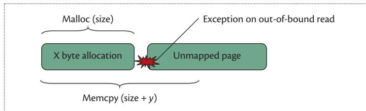
**Figure 4.** Debug heap. A special memory allocator can place each valid memory allocation next to an invalid allocation so that overreads or overwrites of even a single byte are caught instantly.
