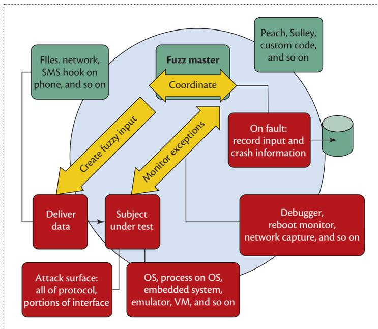
**Figure 3.** Fuzzing overview. Malformed input is created and sent to a program, which is being monitored by a debugger, with results being collected if a crash is found.
