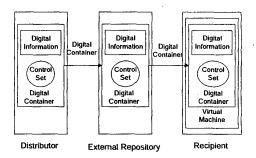
Figure 7. Embedded Control Architecture with External Repository (EC2)
