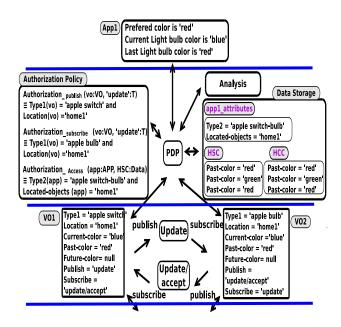
Fig. 4. Using ABAC to control virtual objects communications
