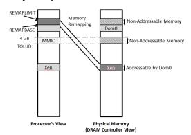
Figure 4: Memory remapping during attack on Q35 chipset.
